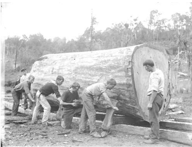
LEFT: FOUR MEN USE TIMBER JACKS TO SHIFT A HUGE LOG. THE TIMBER JACK WAS A NEW ZEALAND ADAPTATION OF THE SCREW JACK, AND WAS WIDELY USED IN THE BUSH WHEN OTHER METHODS OF MOVING LOGS WERE UNAVAILABLE. THE JACK HAD A SPEAR-SHAPED BAR FITTED INTO A STOCK, WHICH CONTAINED A RATCHET OPERATED BY A SYSTEM OF COGS. TURNING A HANDLE MOVED THE BAR UP OR DOWN. ONE END OF THE JACK WAS HELD ON THE GROUND, WHILE THE SPEAR END OF THE BAR WAS FITTED UNDER THE LOG. THE HANDLE WAS THEN TURNED CLOCKWISE TO MOVE THE BAR UP AND ROLL THE LOG SIDEWAYS
